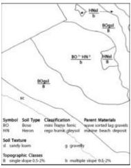
The soils of the South Campus lands consist of two orders: Podzolic and Gleysolic. The Podsolic Order is represented by the Bose Series, a Mini Humo-Ferric Podzol. The Gleysolic Order is represented by the Heron Series, a Rego Humic Gleysol (McBride, 1975).
